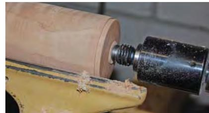
Mount the barrel in the chuck and true up the barrel to remove any wobble. Dish out the bottom of the barrel by ¼". Use a ½" bit to drill the hole that will hold the peg on the handle.
