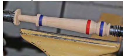
Once the handle is completed, mount the barrel blank between centers and turn it down to round and turn a tenon on one end that matches the size and shape of your chuck. My chuck has dovetail jaws. You don't need a mechanical chuck. You can turn a jam chuck into a block mounted on a faceplate to hold the tenon.
