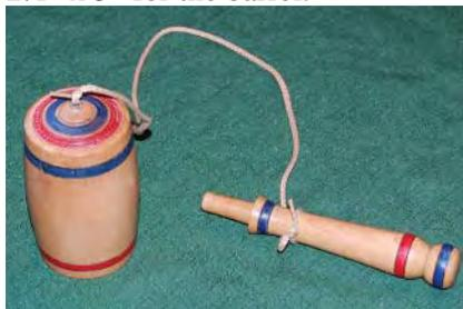
Start by turning the handle between centers. The only critical dimension is for the peg end of the handle. I use a ½" open-end wrench to get the diameter of the peg. Note that the peg is slightly tapered.
