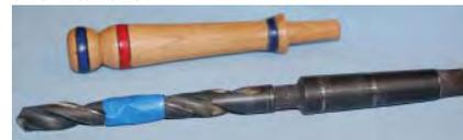
You can use a Jacobs chuck to hold the bit, or you can drill the hole with a ½" bit with a #2 Morse taper. Note the precision measurement tape on the drill bit.
