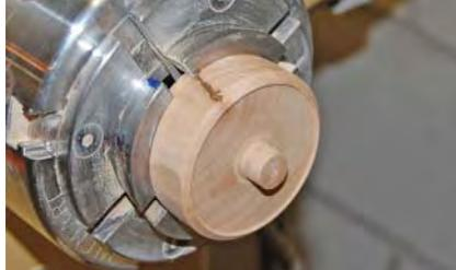
Use the tailstock to hold the barrel in the jam chuck. Using a chatter tool, put some decorations on the top of the barrel and color them with waterproof markers. After removing the barrel from the lathe, remove the nub at the tailstock end with sandpaper and finish the barrel.
