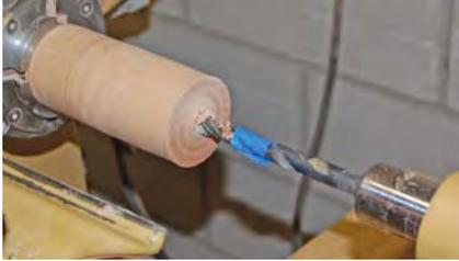
Finish turning the barrel shape and sand from 80 to 320 grit. Use a skew and KC Wire Burners to put lines on the barrel for adding color bands or other decorations. At the chuck end, start the top of the barrel. Leave enough material in the chuck end for making a jam chuck that can be used for the final finish of the top of the barrel. Use the handle to ensure that the hole in the barrel is long enough to let it rest on the shoulder of the handle.
