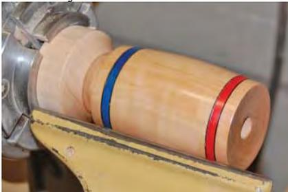
Part off the barrel, giving it a convex shape that matches the concave shape of the bottom of the barrel. I prefer to use a skew to do the parting because
