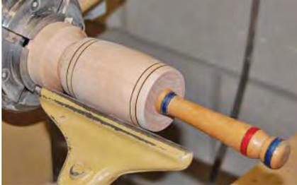
Here is the finished barrel, except for the top. I have put on the bands with waterproof markers and have sealed the surface and applied HUT Crystal Coat.
