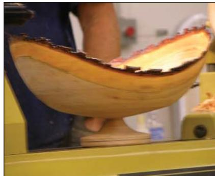
the pedestal base to about 1" thick. When the shape of the pedestal is satisfactory and the underside of the pedestal is hollowed to ½" thick, sand the outside of the bowl and pedestal with 120, 180, and 220 grits. Apply a coat of lacquer and dry the piece for approximately 4 weeks.
