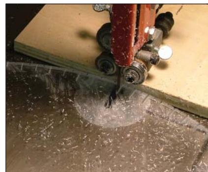
into the edge of my index wheel. For the first series of cuts, the stop was ¼" from the back of the blade. For the remaining set of slots, the stop was positioned right at the back of the blade so there was a significant visible difference in size between the slots.
