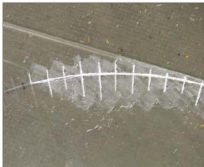
square. I downloaded a grid from <http://www.smithart.us/download.htm> and began. I placed the grid under the Plexiglas, marked the center point, and with a pair of dividers drew a 20" diameter circle. Then using an awl and a metal ruler, I proceeded to transfer the segments from the grid to the circle I had drawn. First 60, then 120, then 240 segments.
