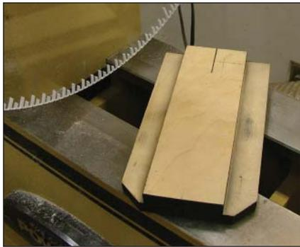
piece was cut two inches wider to provide the sliding surface. Because I keep the ways of my lathe waxed, the plywood carrier slid smoothly without any other surface preparation. I painted the top and sides of the carrier with flat black spray paint. All that was left then was to insert the aluminum stop into the slot in the plywood
