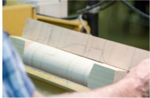
(e.g., beads, coves, v-cuts, shoulders, etc.). They then pre-set a number of calipers to match the various measurements. The storyboard is used to transfer the key points of the design components to the blank and the calipers used to ensure the key points are cut to the correct depth. After rough turning the blank to the approximate shape of the design, Gene used cardboard templates of the design to ensure the various components were precisely replicated.
