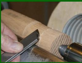
**Skew Chisel, 3/4":** The surface of the cylinder will be smoother when a skew is used to make the cuts rather a spindle gouge. However, there are specific cutting techniques that must be learned in order to use a skew successfully. A skew has two bevels and is available in various configurations—usually slight, or with a gentle curve. It is usually ground at a 45° angle to the side of the tool.
