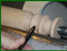
**Spindle Gouge, 3/8":** A spindle gouge, sometimes called a shallow fluted gouge, is used to cut the detail features like concave curves or coves, convex curves or beads, and variations of these cuts. A spindle gouge is usually ground into a shape that looks like a "lady's fingernail", where the sides of the tip area are ground back. This makes the tool more versatile. Various bevel angles are often ground on them but I suggest using a 35° angle to start.
