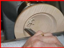
**Bowl Gouge, 1/2":** A bowl gouge is generally used to form both the inside and the outside surfaces of a bowl or platter. It can be used to cut deeper coves when turning spindles. The base side of the bowl blank is fastened to a faceplate with screws and the bowl surfaces are shaped with a bowl gouge. The bowl gouge is probably the most used tool in a turner's tool kit. It is also the tool that has the most variations in the shape and grind configuration of all woodturning tools.
