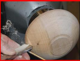
**Square End Scraper, 3/4" wide by 1/4" thick:** The square-end scraper is used to remove the tool marks from the outside surface of the bowl by using the reverse rake technique and scraping the wood directly at a 90° angle. The handle of the scraper will have to be continuously moved or a flat spot will appear on the surface.
