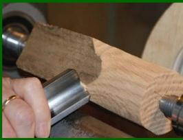
**Spindle Roughing Gouge, 1 to 1-1/2" wide:** A spindle roughing gouge is used for roughing out a blank that is held between a drive center in the headstock and a live center in the tailstock from its original square shape to a rounded cylinder. It can also be used for cutting shallow coves in the spindle's surface. The side cutting edge of a sharp SRG where those parts of the tool are ground flat can be used almost like a skew to create a smooth surface on the cylinder.
