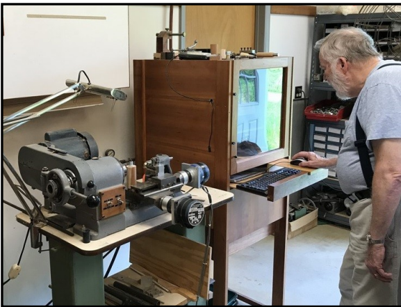
J.R. turning a shaving brush handle on his CNC adapted metal lathe.
