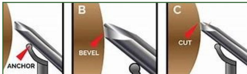
**Anchor:** Set the tool firmly on the tool rest. The forces of the cut must be taken by the tool rest in as direct a manner as possible.
