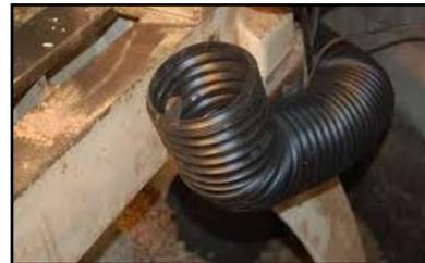
Attaching a hose to the bed of the lathe with a large magnet.
