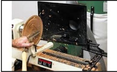
Large commercially made dust hood hooked up to a dust collection hose.
